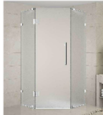
Aston's Neoscope GS frameless neo-angle shower enclosure with integrated two-tier glass shelving is available in frosted glass. Offered in width and length sizes from 34" to 42", it stands 72" high and is made from 10mm ANSI-certified tempered glass and 304-grade stainless steel hardware. Circle No. 164 on Product Card
