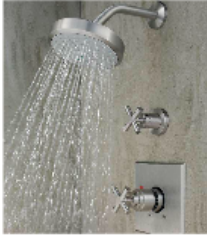
Newport Brass' thermostatic shower mixer and flow control valves are constructed of solid brass and available in 27 finishes. The temperature-adjust handle has a safety stop and index showing the desired temperature. The multi-function showerhead features rubber nozzles and includes five spray modes. Circle No. 156 on Product Card
